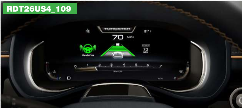
Tungsten 12-inch digital Driver Information Display (DID) cluster.
